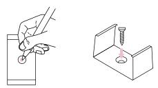
2. Press one edge of channel into mounting clip. Press other edge of channel into mounting clip.
