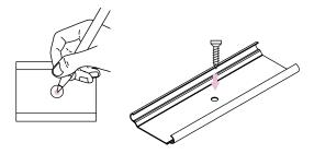
2. Press one edge of channel into mounting clip. Press other edge of channel into mounting clip.
