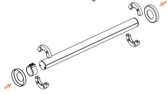
4. Attach upper rings on each side and secure.
