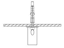
14. The ceiling installation is now prepared. Using the previously assembled components, put the threaded gripper through the mounting sleeve. Ensure that the steel cable shows through the hold of the mounting sleeve.
