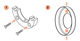
Slide the fixed support bracket and the covers onto the fixture rod. Rest the rod on the mounted rings.
