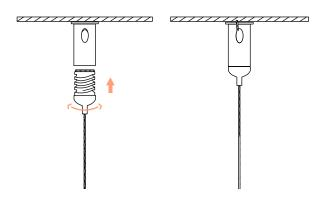
15. Adjust to the desired length by pulling the steel cable. Cut the steel cable excess using pliers or scissors.
