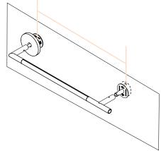
Remove the pre-assembled fixture. Screw the intermediate canopy mount to the drywall with standard drywall screws.
