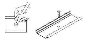
2. Press one edge of profile into mounting clip. Press other edge of profile into mounting clip.
