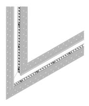
Secure powered corner cover with hex screws provided.
