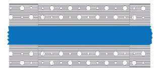
Cover the wings of the fixture with thin drywall tape.
